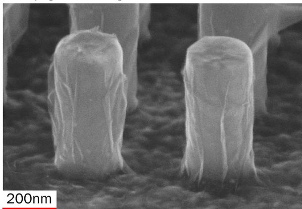
Fig. 2 SEM image of nanowire exhibiting a loose carbon sheet covering the entire wire and extending to the adjacent wires.
