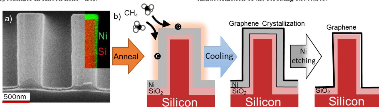
Fig. 1 Nanowire shaped graphene growth method. a) SEM image of nickel deposited on silicon nanowires with inset TEM-EDS image showing nickel and silicon layers. b) example process in which methane is decomposed on nickel during annealing to form graphene sheets that remain on the SiO<sub>2</sub> surface of Si nanowires after Ni etching.
