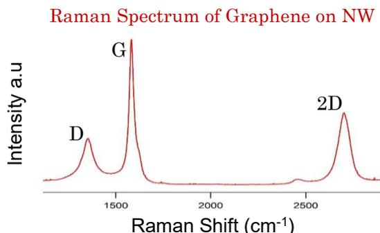
Fig. 3 Raman micro-spectrography results obtained from the sample in fig.2. The carbon G peak at ~1580cm<sup>-1</sup> and 2D peak at ~2700cm<sup>-1</sup> relate to the graphene structure. The carbon D peak at ~1350cm<sup>-1</sup> is related to defects in the graphene layer.
