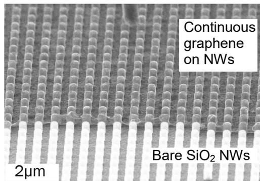
Fig. 4 SEM image of nanowire array covered in a large continuous carbon sheet. The sheet has been peeled off in the lower section of the image to show the contrast with the insulating SiO<sub>2</sub> wires.
