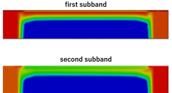
Fig. 5 Two dimensional electron concentration distribution of the first and the second subbands. There are two peaks of concentration along the depth of the second subband electron. Color indicates logarithmic scale of concentration from  $10^{10}$  to  $10^{20} \text{ cm}^{-3}$ .
