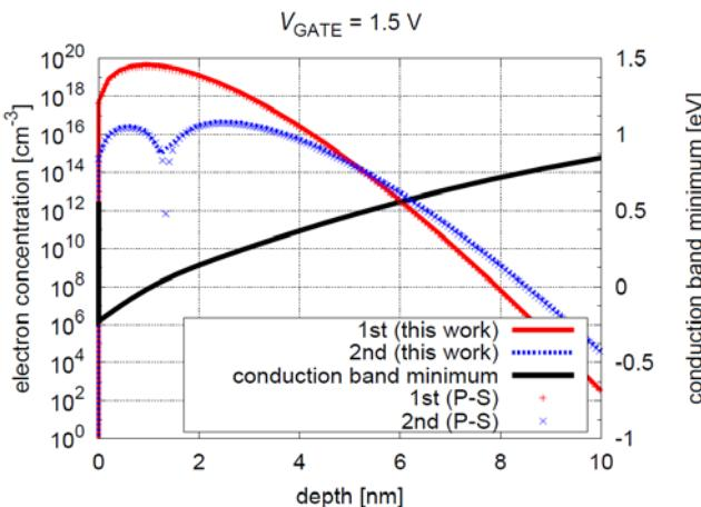
Fig. 4 Electron concentration depth profile at the channel center. The black line shows the conduction band minimum and Poisson-Schrodinger results are shown with markers. The results of the first and the second subbands of the proposed method are shown by the red and the blue line almost identical to Poisson Schrodinger ones.
