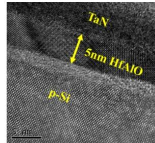
Fig. 1 HRTEM cross-section image of 5nm-thick HfAlO<sub>x</sub> NCFET.
