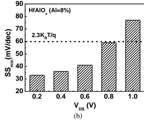
Fig. 4 (a)  $I_{DS}$ - $V_{GS}$  and (b)  $SS_{min}$ - $V_{DS}$  characteristics of 5nm-thick  $\text{HfAlO}_x$  NCFET with 8%-Al doping.
