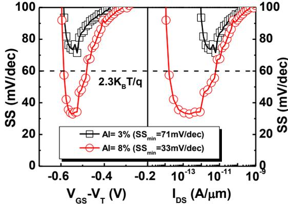
Fig. 3  $SS$  as the function of gate overdrive voltage ( $V_{OV}$ ) and  $I_{DS}$  of 5nm-thick  $\text{HfAlO}_x$  NCFET with 3% and 8% Al doping.
