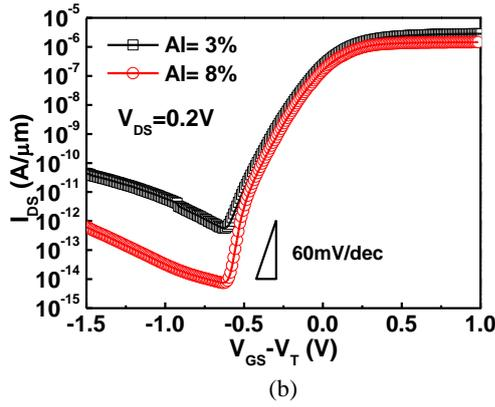
Fig. 2 (a) Output  $I_{DS}$ - $V_{DS}$ , and (b) transfer  $I_{DS}$ - $V_{GS}$  characteristics of 5nm-thick  $\text{HfAlO}_x$  NCFET with 3% and 8% Al doping.
