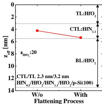
**Fig. 4.** The effect of Si SAF on  $Z_{\text{eff}}$ .
