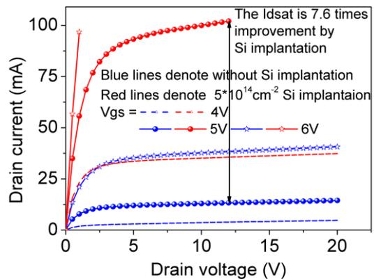
Fig. 6. Id-Vds of Si implanted DMOSFET compared with non-Si implanted baseline. Increase in saturation current is observed. The Idsat of Si implanted DMOSFET at  $V_{gs}=5V$  is 7.6 times larger than that of the baseline one.
