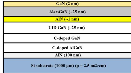
Fig. 1 Cross-sectional view of the AlGaN/AlN/GaN HEMTs grown on the extremely-low resistivity silicon substrate.
