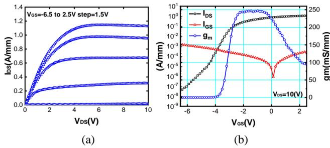
Fig. 3 (a) Measured DC  $I_{DS}$ - $V_{DS}$  characteristics of the 100-nm AlGaIn/GaN HEMT on ELR Si substrate ( $W_G = 2 \times 12.5 \mu\text{m}$ ) with a good pinch-off and high output resistance. (b) Transfer characteristics at  $V_{DS}=10\text{ V}$ .
