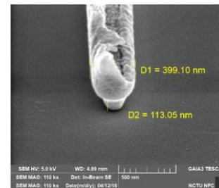
Fig. 2 FIB micrograph of T-gate for the fabricated GaN HEMT.
