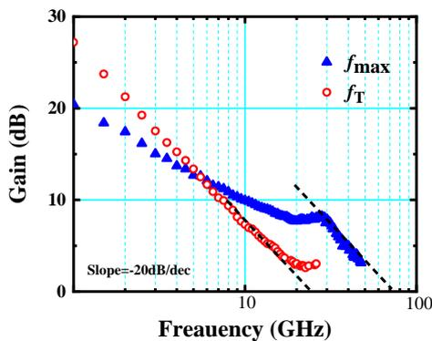
Fig. 4 Measured frequency response of the fabricated GaN HEMT on the ELR Si substrate at  $V_{DS} = 10\text{ V}$  and  $V_{GS} = -3.5\text{ V}$ . The extracted  $f_T$  and  $f_{max}$  are 27 GHz and 71 GHz, respectively.
