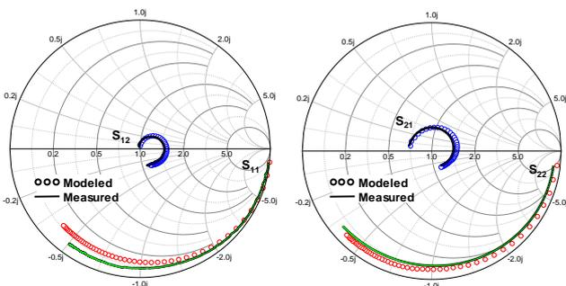
Fig. 5 Measured and modeled frequency response of the fabricated GaN HEMT at  $V_{DS} = 10\text{ V}$  and  $V_{GS} = -3.5\text{ V}$ . The extracted  $f_T$  and  $f_{max}$  are 27 GHz and 71 GHz, respectively.
