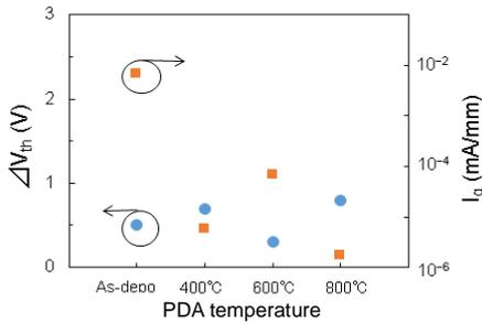
Fig. 3 Dependences of the  $\Delta V_{th}$  and the  $I_g$  at a  $V_g$  of  $4.7$  V on the PDA temperature.
