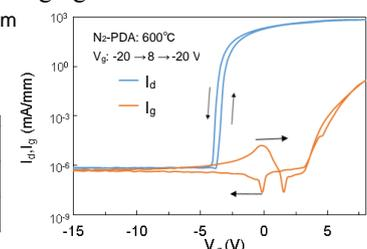
Fig. 2 Typical result of the transfer curve measurements. The PDA temperature was 600°C.
