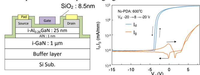
Fig. 1 Schematic cross-sectional view of the SiO<sub>2</sub>/AlGa<sub>0.26</sub>N/GaN MIS-HEMT.
