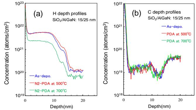
Fig. 5 SIMS depth profiles for ALD-SiO<sub>2</sub>/AlGaIn ( $15/25$  nm) layers, (a) H, (b) C.
