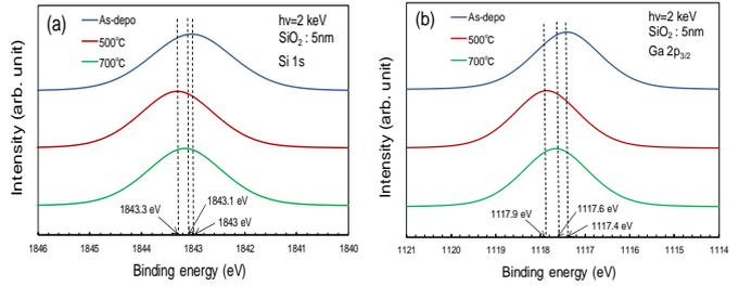
Fig. 4 XPS core-level spectra obtained from SiO<sub>2</sub>/AlGaIn ( $5/25$  nm) layers, (a) Si 1s, (b) Ga  $2p_{3/2}$ .
