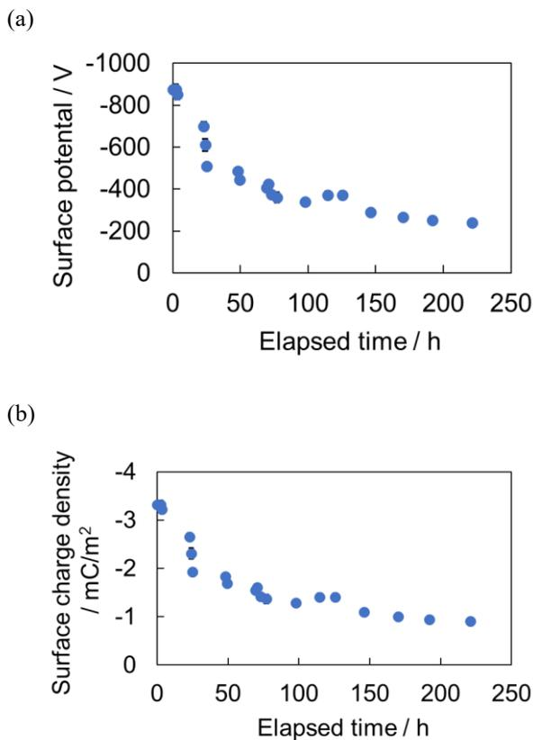
Fig. 3. Time-dependent of (a) surface potential and (b) surface charge density for poly(HNA/HBA) electrets used in this study.
