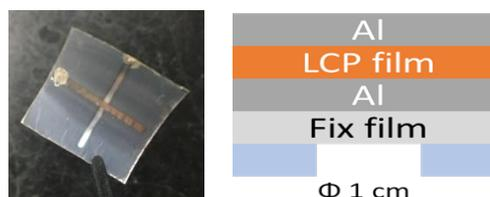
Fig. 2. (left) A photograph of poly(HNA/HBA) film with electrodes. (right) A moonie type device structure for inverse piezoelectric measurement.
