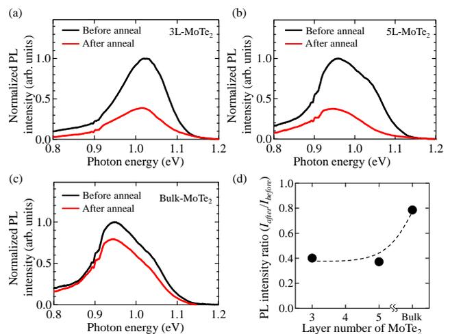
Fig. 1 PL spectra before and after thermal annealing for samples with (a) 3L-, (b) 5L-, and (c) bulk-MoTe<sub>2</sub> on SiO<sub>2</sub>. (d) A ratio of integrated PL intensities between before and after thermal annealing plotted as a function of the layer number.
