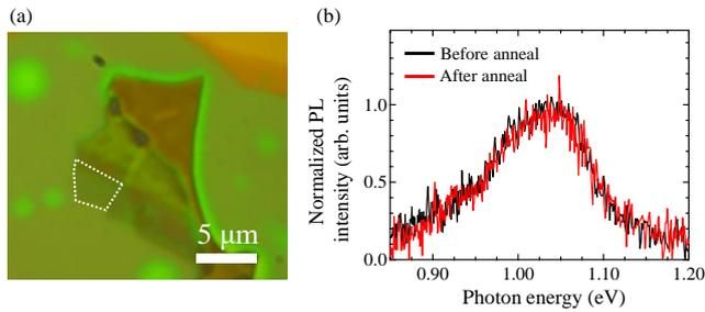
Fig. 2 (a) An optical microscope image and (b) PL spectra before and after thermal annealing for a 3L 2H-MoTe<sub>2</sub> encapsulated by hBN.
