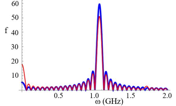
Fig. 1 Fourier function against a frequency. Here, we set parameters as  $\lambda_1/2\pi=1$  GHz,  $g/2\pi=0.5$  GHz,  $\omega_1/2\pi=0.2$  GHz,  $\omega_2/\omega_1=1.2$ ,  $g'/g=2.1$ ,  $\lambda_2/\lambda_1=10.7$ ,  $L=2$ ,  $N=10000$ ,  $t_{min}=0$ , and  $t_{max}=100$  ns. Also, we set  $T=150$  (75) ns for the blue (red) plot.
