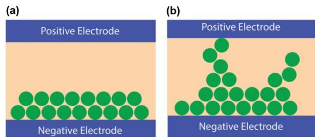
Fig. 1: The conducting channel formalism illustrated by a charged species cluster model. (a) illustrates the pristine preformed state. (b) illustrates a possible formed state, showing one complete conducting channel forming a continuous path between the negative and positive contacts. The green circles represent discrete charged species, hosted by a dielectric, shown in tan [7].
