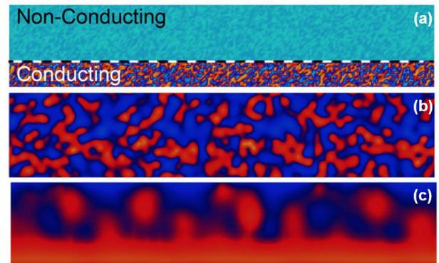
Fig. 3: (a) illustrates the pristine dielectric thin-film structure, (b) and (c) show two snapshots representing a transient stage and the final stage, respectively, of irreversible electroformation [7].
