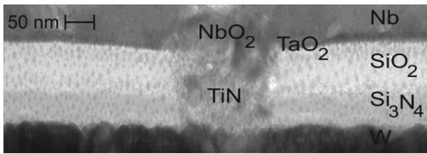
Fig. 2: Analytical TEM cross-sectional image of the self-assembled monolithically integrated NbO<sub>2</sub> selector self-aligned to a TaO<sub>2</sub> memristor after electroforming, with approximate locations of material boundaries. The TiN via is 75nm in diameter and is axially symmetric [6].
