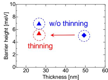
Fig.4. Thickness dependence of the energy barrier for samples without thinning ( $\blacktriangle, \blacklozenge$ ) and after thinning of 50-nm-thick grown film ( $\blacktriangle$ ).
