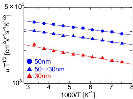
Fig.3. Arrhenius plot of  $\mu T^{1/2}$  for samples without thinning ( $\blacktriangle, \blacklozenge$ ) and after thinning of 50-nm-thick grown film ( $\blacktriangle$ ).
