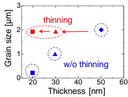
Fig.2. Thickness dependence of grain size for samples without thinning ( $\blacksquare, \blacktriangle, \blacklozenge$ ) and after thinning of 50-nm-thick grown films ( $\blacksquare, \blacktriangle$ ).
