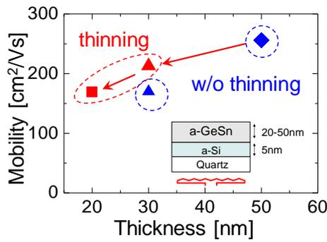
Fig.1. Initial sample structure and thickness dependence of carrier mobility for samples without thinning ( $\blacktriangle, \blacklozenge$ ) and after thinning of 50-nm-thick grown films ( $\blacksquare, \blacktriangle$ ).
