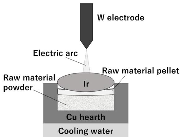
Fig. 1 Schematic of the CH method
