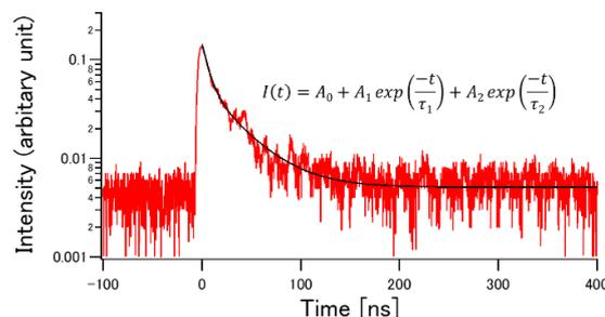
Fig. 4 Decay time profile of Ce doped CaHfO<sub>3</sub>
