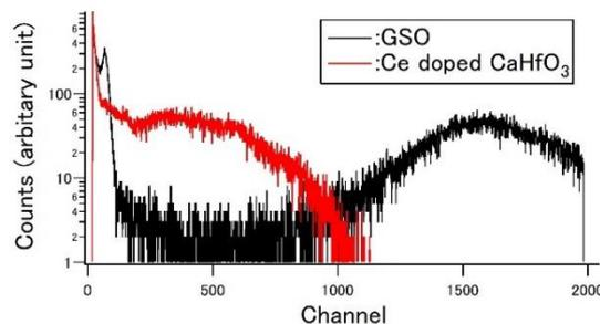
Fig. 5 Pulse height spectra of Ce doped CaHfO<sub>3</sub> excited by a <sup>241</sup>Am source
