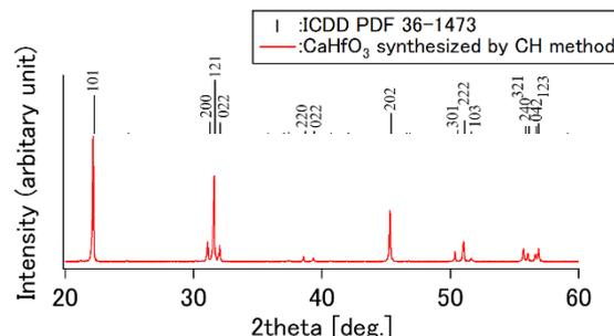
Fig. 3 Powder X-ray diffraction pattern of Ce doped CaHfO<sub>3</sub> synthesized by CH method
