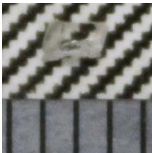
Fig. 2 Photograph of Ce doped CaHfO<sub>3</sub> synthesized by CH method
