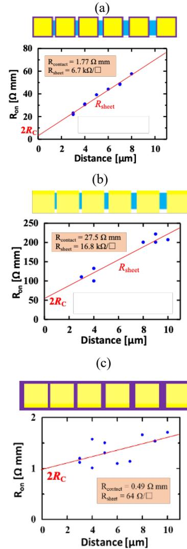
Fig.4 Results of TLM measurements (a) with 2DHG and boron-doped layer (b) only 2DHG without boron-doped layer (c) with only boron-doped layer
