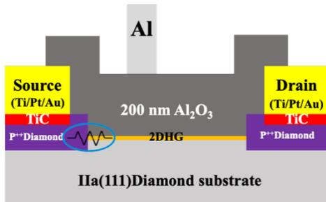
Fig.1 The sectional view of boron-doped diamond MOSFETs
