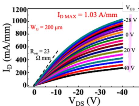
Fig.3 The drain current density ( $W_G = 200 \mu\text{m}$ ,  $V_{DS} = 0$  to  $-40$  V,  $V_{GS} = -28$  to  $40$  V)
