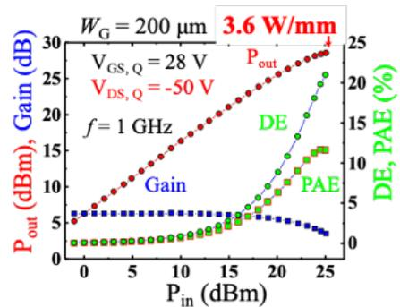
Fig.5 The large signal performance ( $W_G = 200 \mu\text{m}$ ) This work is supported in part by MEXT Project on Design & Engineering by Joint Inverse Innovation for Materials Architecture.
