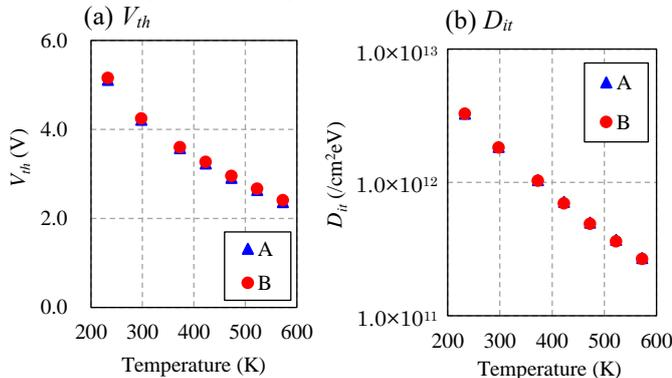
Fig. 3. The temperature dependence of (a)  $V_{th}$  and (b)  $D_{it}$ .
