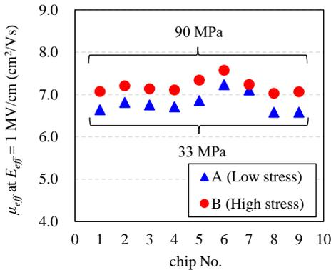
Fig. 2.  $\mu_{eff}$  at  $E_{eff}=1$  MV/cm at 298K was plotted. Chip No. corresponds to the position on the wafer.
