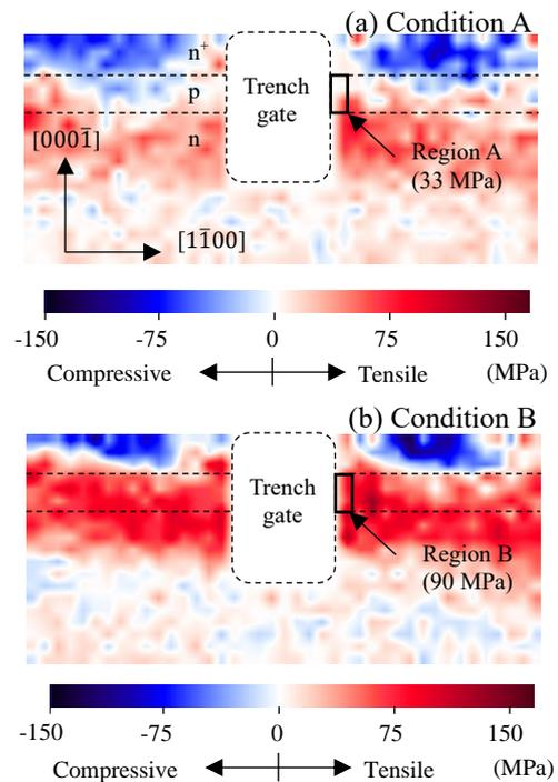
Fig. 1. The stress toward [1 $\bar{1}$ 00] mapping images of cross-sectional trench MOSFETs in which polycrystalline silicon was fabricated under condition A (a) and B (b). The average of the stress in regions A and B is shown.
