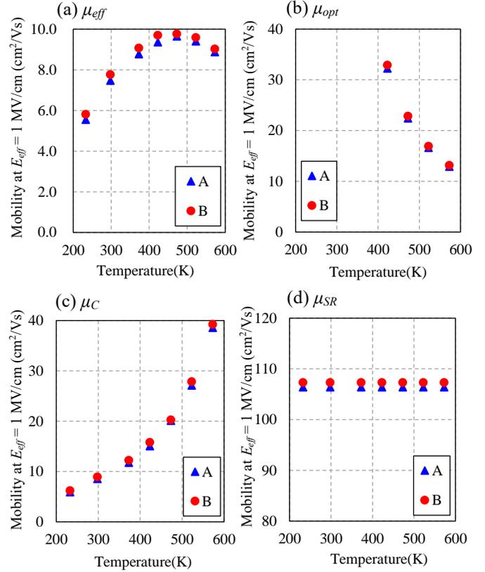
Fig. 4. The scattering mobility values were calculated from the temperature dependence of  $\mu_{eff}$ . Each mobility at  $E_{eff}=1$  MV/cm was plotted. (a)  $\mu_{eff}$ , (b)  $\mu_{opt}$ , (c)  $\mu_C$  and (d)  $\mu_{SR}$ .
