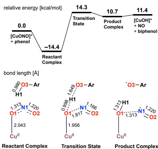
Figure 1. Energy diagram for the nitrite reduction and optimized geometries of RC, TS, and PC.
