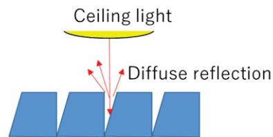
**Fig. 4. Diffuse light caused at the groove of the DCRA.**
