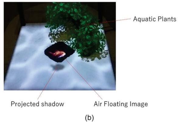
**Fig. 7. Air floating image with projection mapping.** (a) is side view of the arrangement. (b) is picture of the prototype.
