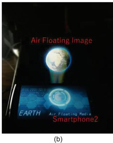
**Fig. 6. Air floating display system using two smartphones**
