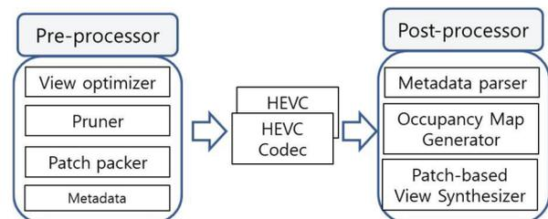
Fig. 1 (a) Architecture of 3DoF+ video compression, (b) block diagrams of preprocessor/postprocessor
