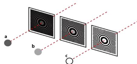
Fig. 1 Light intensities of the object points reconstructed from BW-CGHs
