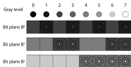
Fig. 2 Assignment of the object points of the 3D object to the bit planes consisting of BW-CGHs with different gray levels
