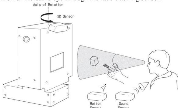
Figure 1. Schematic of the interactive holographic display.
