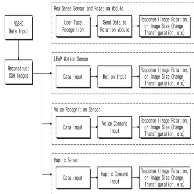
Figure 2. Pipeline of the holographic display system based on user's interactive sensing information.
