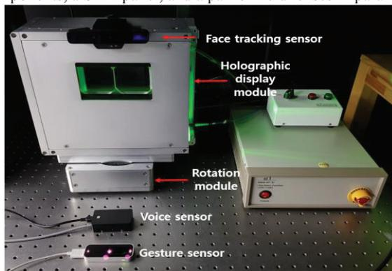
Figure 4. Experimental setup of our system.
