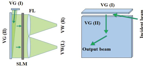
Figure 3. Configuration of the backlight unit for the holographic display module that comprises two thin backlight components, a SLM panel, and a pair of field lenses in parallel.
