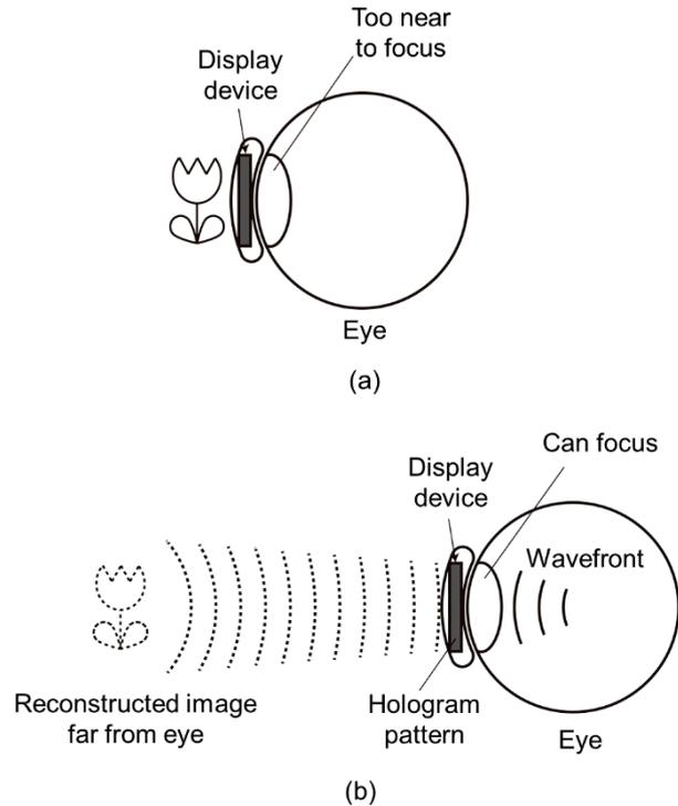
Fig. 1 Image formation for contact lens display: (a) problem using conventional displays, and (b) solution using holographic technique
