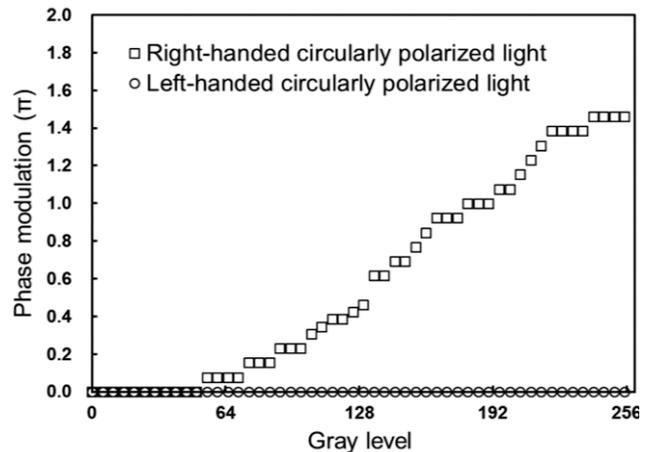
Fig. 4 Measured phase modulation characteristic of the TN-SLM
