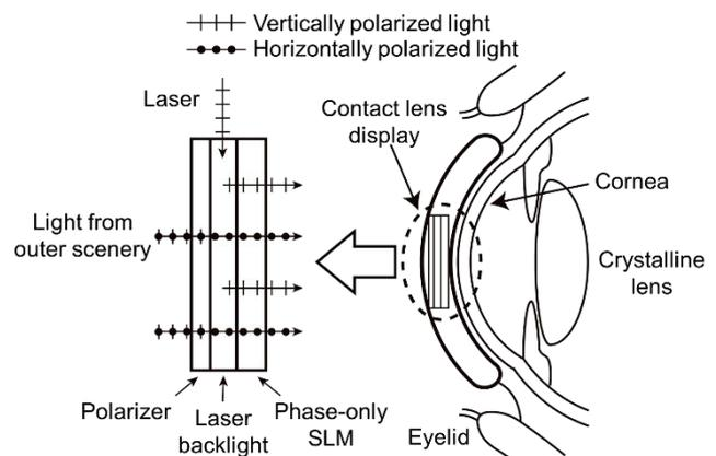
Fig. 2 Structure of holographic contact lens display
