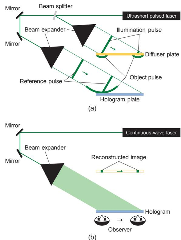
Fig. 1 Schematic diagram of top view of optical setup in LIF holography. (a) Recording. (b) Reconstruction.
