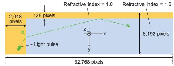
Fig. 3 Schematic diagram of brief situation on diffuser plate in proposed simulation model.
