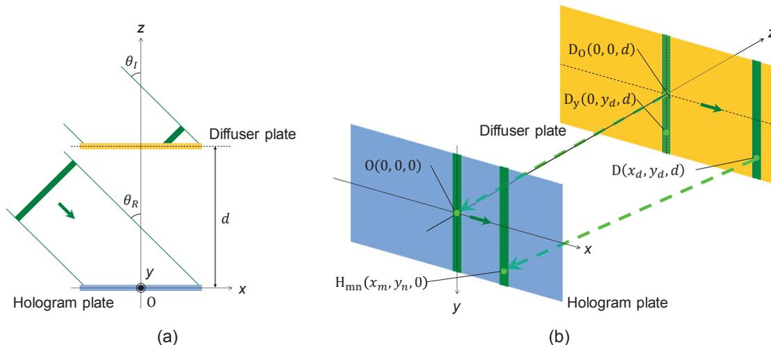
Fig. 2 Schematic diagram of conventional simulation model in LIF holography. (a) Top view. (b) Bird's eye view.
