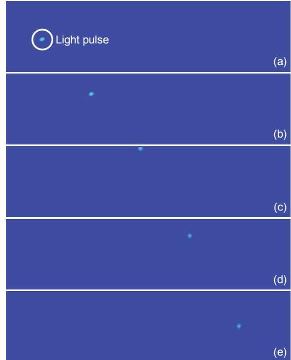
Fig. 4 examples of the intensity distributions in light pulse propagation obtained by FDTD simulation at time steps of (a) 10,000, (b) 23,000, (c) 36,000, (d) 49,000, and (e) 62,000, respectively.
