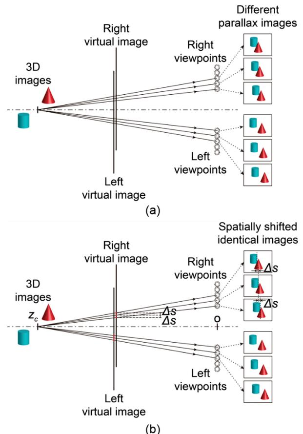
**Fig. 1 Three-dimensional image generation schemes for (a) the conventional SMV HMD and (b) the proposed simplified SMV HMD**
