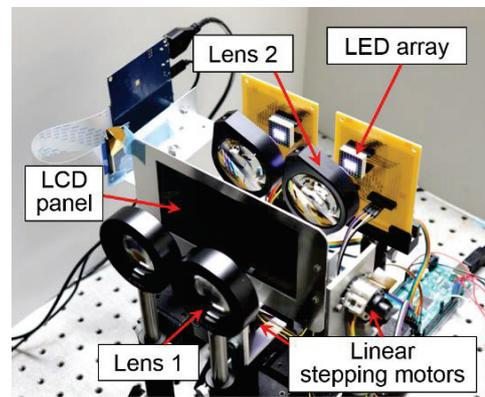
Fig. 3 Photograph of the experimental system
