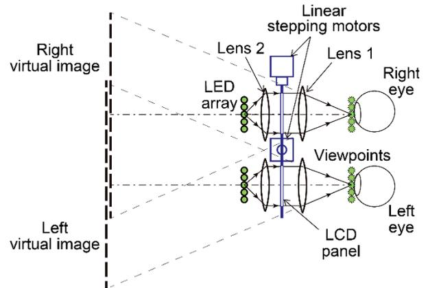
Fig. 2 Schematic of the experimental system for the simplified SMV HMD
