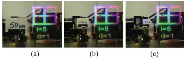
Fig. 9 The retinal images generated by the Maxwellian-view display with white laser backlight which composed of the red, green, blue laser, the camera focus at (a) 50cm, (b) 100cm, (c) 150cm.
