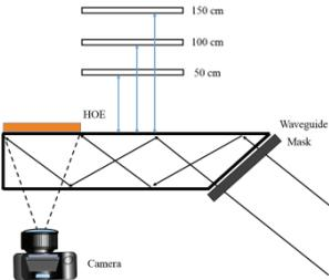
Fig. 4 The recording system. The camera focus at 50 cm, 100 cm, 150 cm behind the waveguide, respectively.
