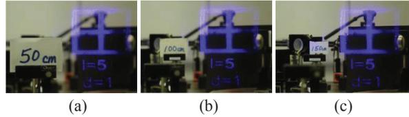
Fig. 8 The retinal images generated by the Maxwellian-view display with blue laser backlight, the camera focus at (a) 50cm, (b) 100cm, (c) 150cm.
