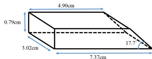
Fig. 2 The information of the trapezoidal waveguide
