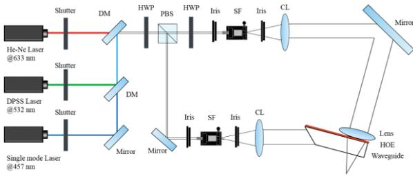
Fig. 3 the system for generating the HOE device. DM: dichroic mirror, HWP: half-wave plate, PBS: polarized beam splitter, SF: spatial filter, CL: collimating lens.
