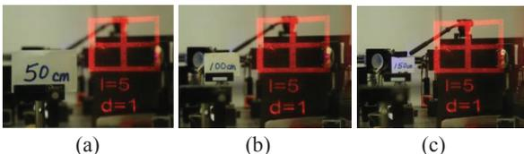
Fig. 6 The retinal images generated by the Maxwellian-view display with red laser backlight, the camera focus at (a) 50cm, (b) 100cm, (c) 150cm.
