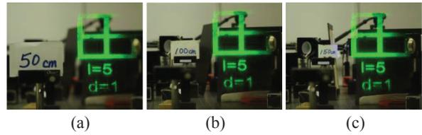
Fig. 7 The retinal images generated by the Maxwellian-view display with green laser backlight, the camera focus at (a) 50cm, (b) 100cm, (c) 150cm.
