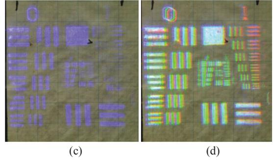
**Fig. 13** The USAF test target generated by the Maxwellian-view display with (a) red, (b) green, (c) blue (d) white laser backlight
