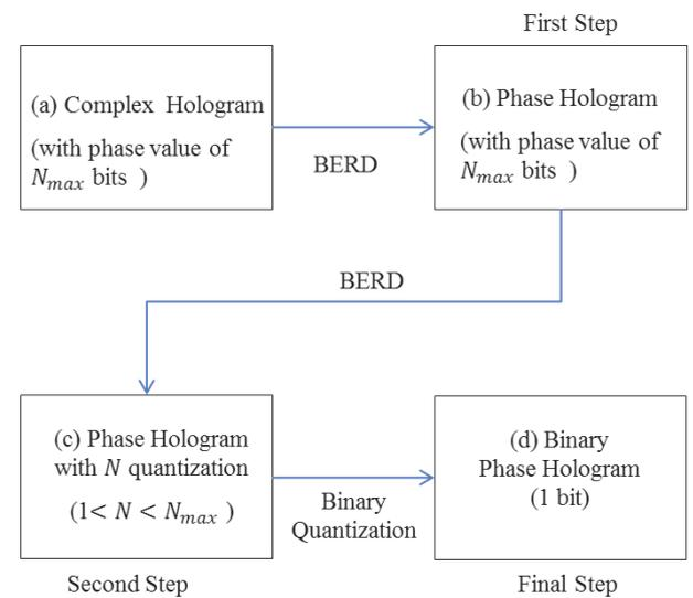
Fig. 2 Algorithm of Three-step binary phase hologram generation
