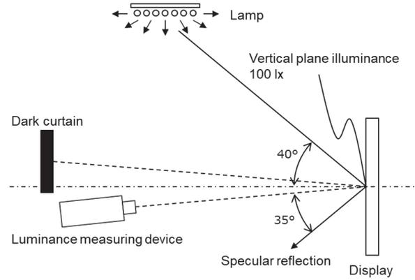
**Figure 10.** ACR evaluation system for a large-scale display
