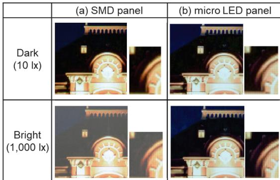
**Figure 9.** Photographs of (a) typical SMD panel and (b) micro LED panel in a dark/bright environments
