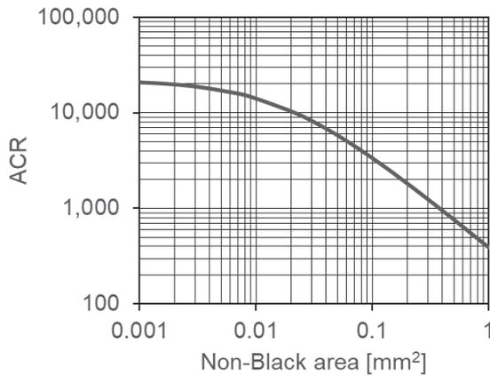
**Figure 11.** Simulated *ACR* relative to non-black area including RGB LEDs
