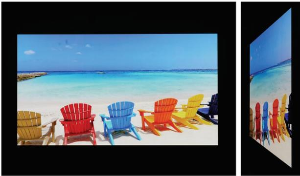
**Figure 5.** Wide viewing angle by using micro LEDs with Lambertian emission pattern
