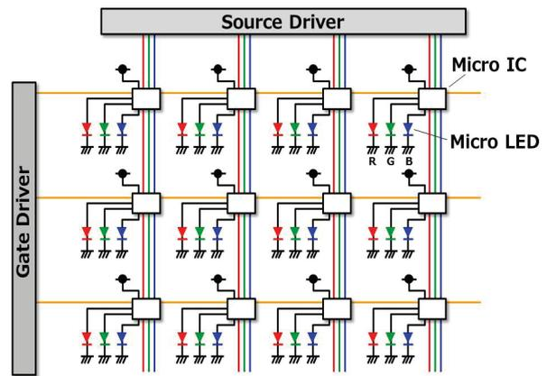
**Figure 6.** Schematic of active matrix driving using RGB micro LEDs and micro IC in each pixel
