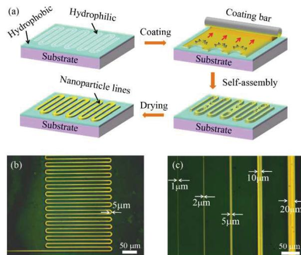
**Fig. 2 Selective Deposition of Metallic Ink**
