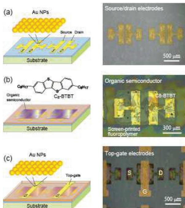
**Fig. 3 Fully-Printed Organic Thin-Film Transistors**
