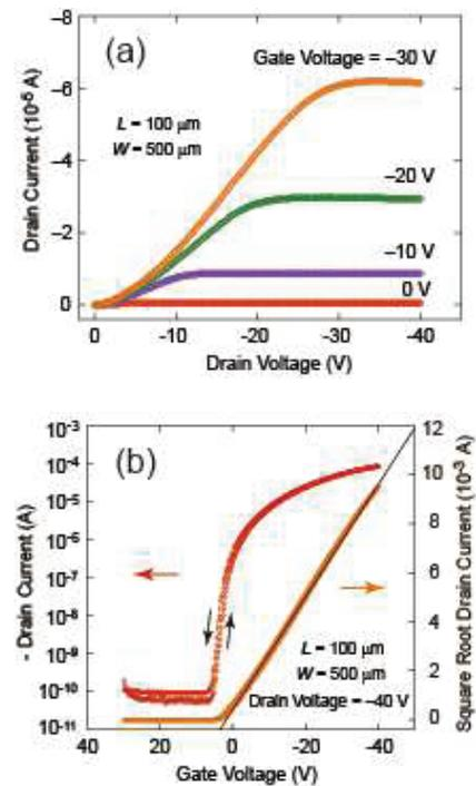
**Fig. 4 Electrical Performance of Fully-Printed Organic Thin-Film Transistors**
