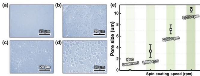
**Fig. 4** (a) Optical microscopy (OM) image of the IGZO films. OM images of POL on the IGZO films prepared at spin-coating speeds of (b) 1000 rpm, (c) 2000 rpm, (d) 3000 rpm. (e) Error bars of pore size denote standard deviations over 5 samples.
