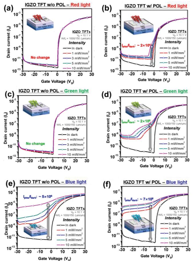
**Fig. 5** Transfer characteristics of IGZO phototransistors without POL under (a) red, (c) green, and (e) blue light illumination at different intensities. Transfer characteristics of IGZO phototransistors with POL under (b) red, (d) green, and (f) blue light illumination at different intensities.
