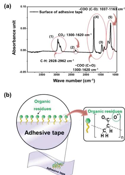
Fig. 3 (a) FT-IR spectroscopy on the surface of adhesive tape and (b) The schematic illustration of poly-acrylate on adhesive tape.
