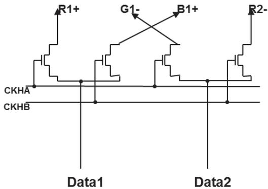
Figure 1. Schematic circuit diagram of 1:2 mux
