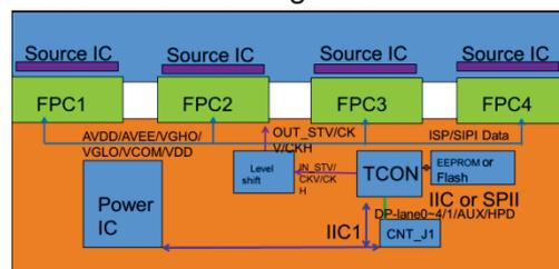
Figure 5. Main block diagram with 4 IC solution
