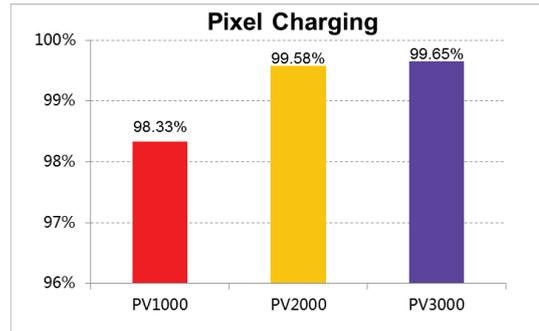
Figure 3. Pixel charging of different thickness of PV
