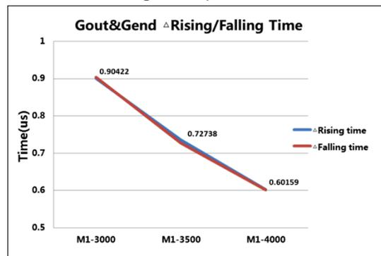
Figure 4. Rising/falling time of different thickness of M1
