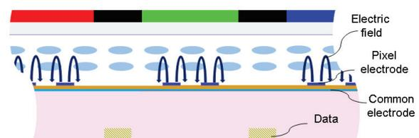
Fig.3 The Electric Field of the Pixel
