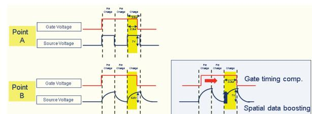
**Fig. 2 Timing and driving ability schematic diagram at Point A and Point B**
