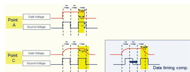
**Fig. 3 Timing and driving ability schematic diagram at Point A and Point C**
