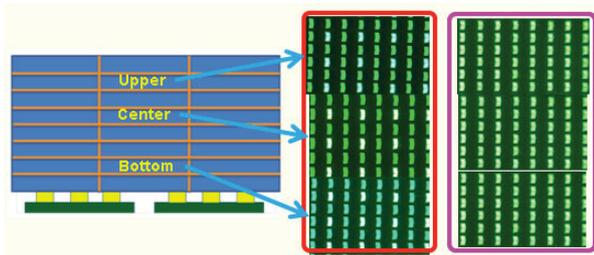
**Fig. 7 visual dash-line elimination by spatial over drive and spatial gain weighting . Visual dash-line like Fig.7a caused by panel architectuer. Fig.7b is the effect applied the spatial over drive and spatial gain weighting .**
