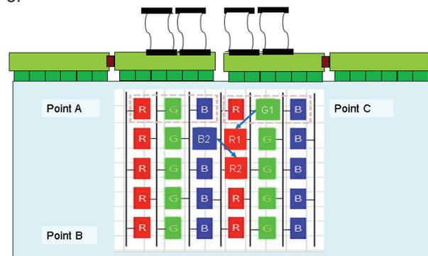
**Fig. 1 1D1G Flip Pixel panel structure**
