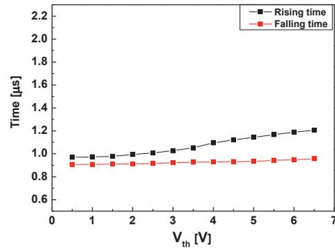
**Fig. 5 The rising / falling time characteristics according to threshold voltage variation**
