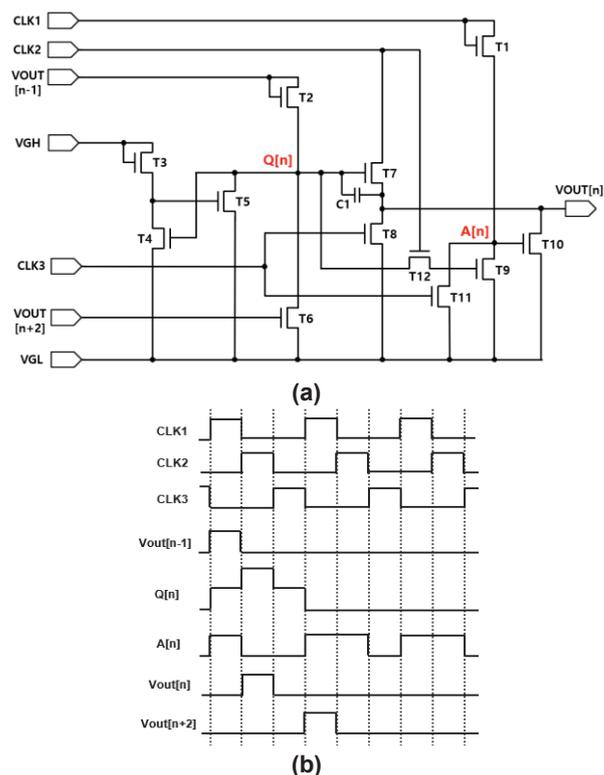
Fig. 1 (a) proposed gate driver circuit (b) timing diagram
