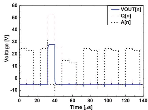
Fig. 3 The simulated waveform of VOUT[n], Q[n], and A[n]
