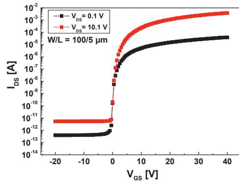
Fig. 2 I-V characteristics of a-IGZO TFT model
