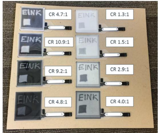
**Fig. 3** The effect of different ink compositions on contrast ratio with magnetic stylus writing from dark and white states.
