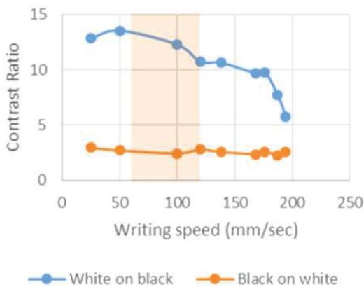
**Fig. 2** Effect of writing speed on contrast ratio with magnetic ink giving electrically-driven white and dark states of 78.4 and 15.6 L\*, respectively. Normal writing speed shown by shaded region. This ink formulation was optimized for white writing on a black background.
