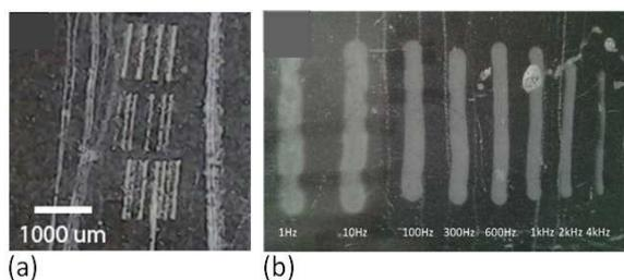
**Fig. 4** Writing onto magnetic film with electromagnetic head. (a) High-resolution lines (width ~100 microns); (b) changing line width by adjusting the frequency of AC current supplied to the electromagnet at a constant voltage.
