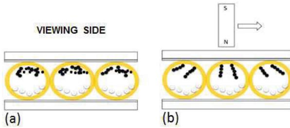
**Fig. 1** Schematic, cross-sectional drawing of E Ink MEP film. (a) Dark state switched electrically; (b) Magnetically-written gray state with chained ferromagnetic black pigment particles
