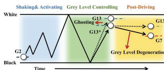
Figure 1. Optical trace of particle in PWM waveform.
