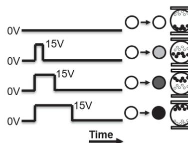
Figure 2. PWM waveform drive EPD.
