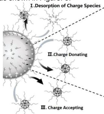
Figure 3. Charging mechanism of EPD.
