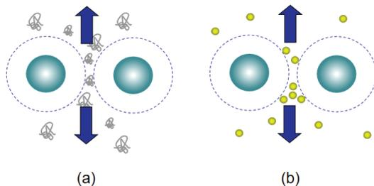
**Figure 9. Depletion Flocculation for Bistability. (a) with free polymers and (b) with nan-particles.**
