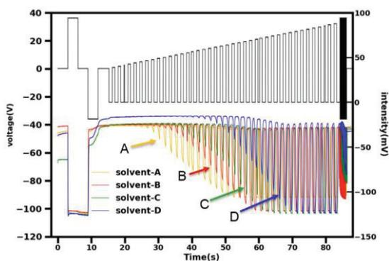
Figure 4. Optical response of various solvent viscosity
