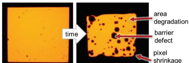
**Figure 1: water induced degradation of flexible optoelectronic devices**
