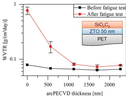
**Figure 6: WVTR of a dual stack ZTO +  $\text{SiO}_x\text{C}_y$  on PET Melinex 401 CW before and after a bending test**
