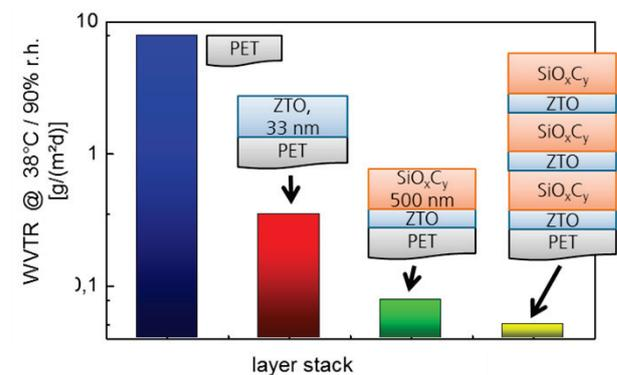
Figure 5: effect of SiO<sub>x</sub>C<sub>y</sub>H<sub>2</sub> coating on ZTO barrier layers
