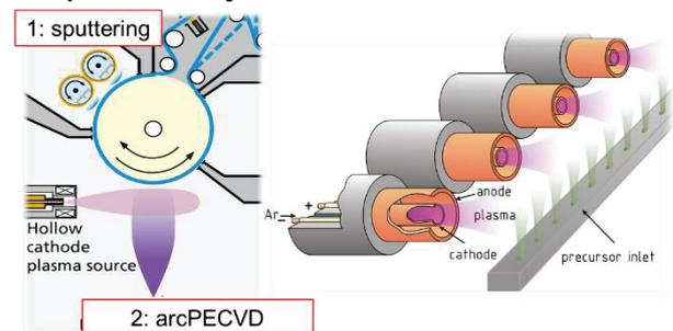
**Figure 3: left: arrangement of sputtering and PECVD source in the *novoFlex*<sup>®</sup> 600 machine; right: array of hollow cathode plasma sources**
