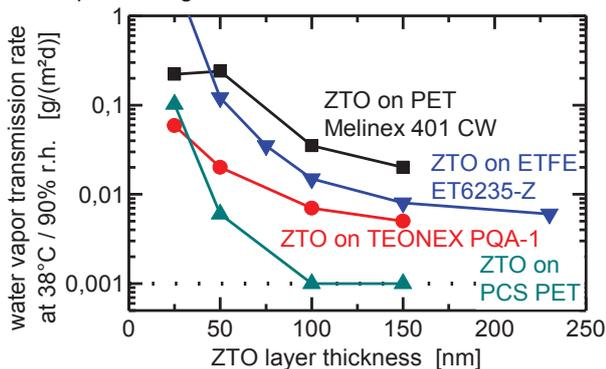
Figure 4. WVTR of ZTO layers on different substrates
