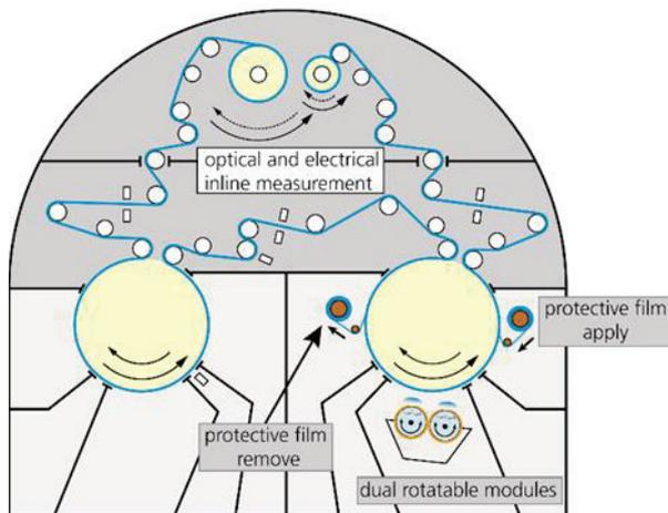
**Figure 2: vacuum roll coater *coFlex*<sup>®</sup> 600 with 650 mm coating width and 6 different deposition stations arranged around 2 process drums.**
