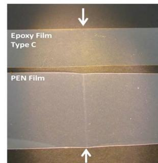
Fig. 4 Epoxy Film after 20k Times of Repeated Bending ( $r=1$  mm)
