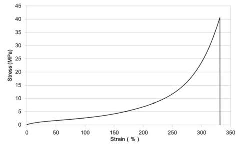
Fig. 7 S-S Curves of Stretchable Epoxy Film
