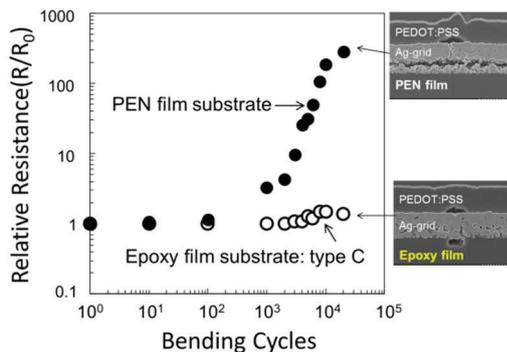
Fig. 12 Comparison of Relative Resistance after Repeated Bending of EL Lighting Device (Epoxy Film Base vs PEN Film Base)
