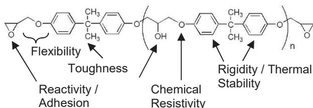
Fig. 1 Generic Structure of Epoxy Resin and its Functional Groups for Various Properties
