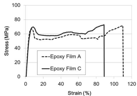
Fig. 3 SS-Curves of High Flexible Epoxy Film
