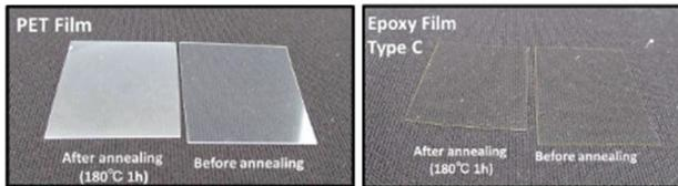
Fig. 5 Comparison of PET Film and Epoxy Film after Thermal Treatment (180°C x 60 min)
