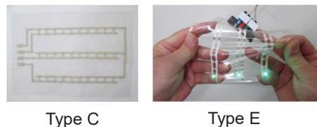
Fig. 9 Ag Nano-Ink Based Printed Conductive Patterns on Epoxy Films
