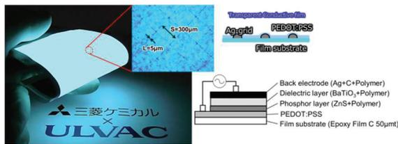
Fig. 11 EL Lighting Device on Epoxy Film (Type C)
