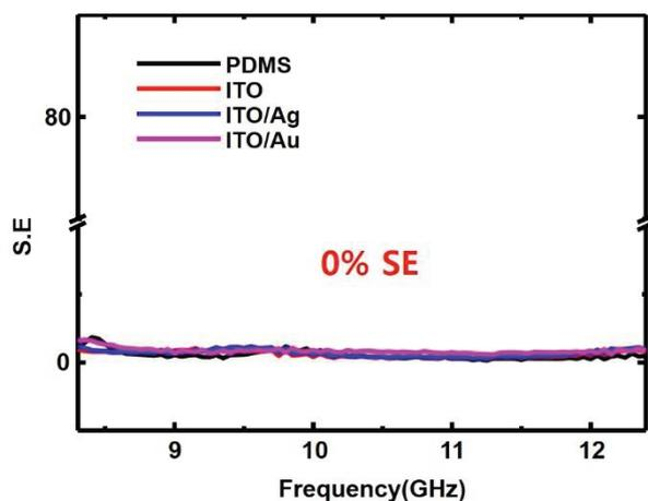
**Figure-4 EMI SE of PDMS membrane which transferred ITO Branch of each condition**
