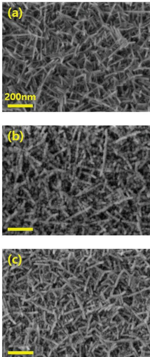
Figure-2 SEM image of (a) ITO branch and (b) ITO branch with Ag nano dot, (c) ITO branch with Au nano dot.
