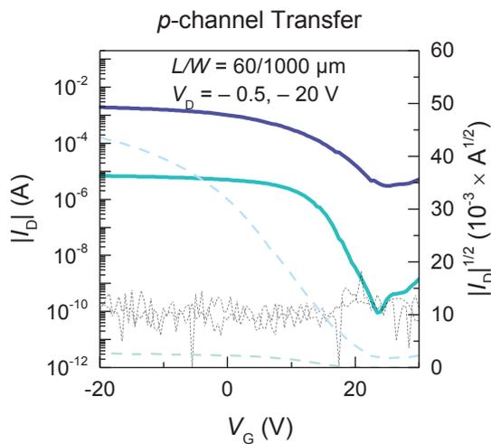
Figure 2. p-channel transfer curve of bottom-gated bottom contact structured SWNT transistor on a rigid substrate.
