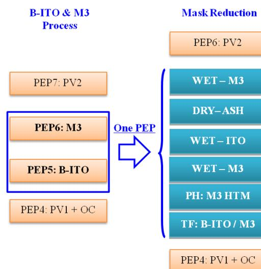
**Fig. 1 Process of mask reduction for VAC-LCD**
