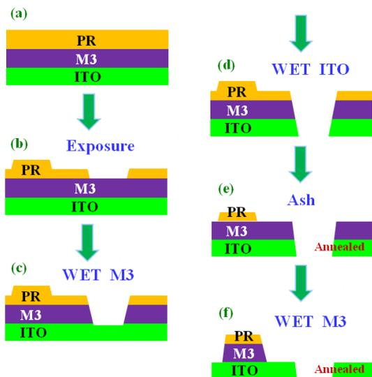
**Fig. 2 Processing details of mask reduction**
