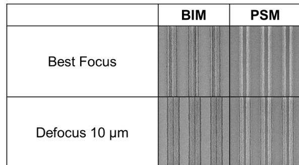
Fig. 8 Comparison of top view images at different focus positions
