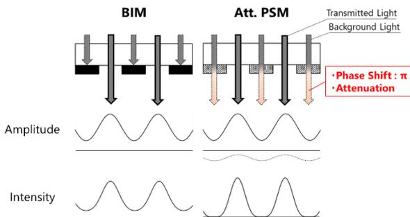
Fig. 3 Principle of resolution enhancement with Att. PSMs
