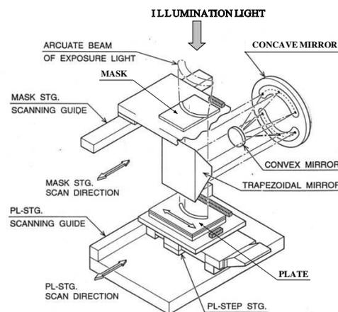
Fig. 1 Configuration of a mirror-projection exposure tool
