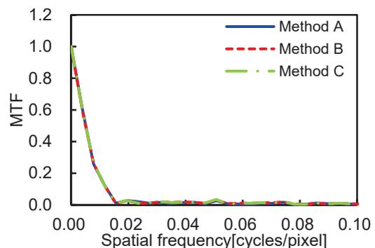
**Fig. 12 MTF curves of aerial image formed by use of AIRR calculating slanted edge method.**
