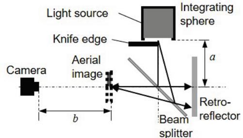
**Fig. 8** Experimental setup to obtain the aerial image of a slanted knife edge.
