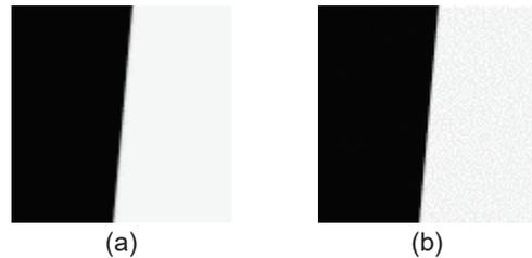
**Fig. 4 Simulated 5-degree-slanted knife edge images (a) without a white noise and (b) with a white noise.**
