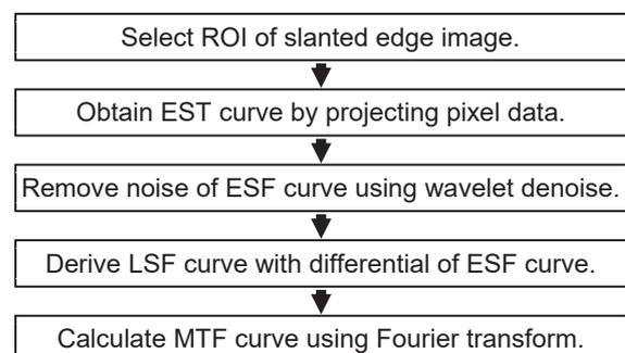
Fig. 2 Slanted edge method for calculating MTF.
