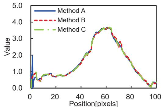
**Fig. 11 LSF curves of aerial image formed by use of AIRR calculating slanted edge method.**
