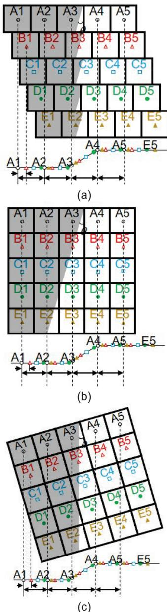
**Fig. 3 Projection method of slanted edge image.**
