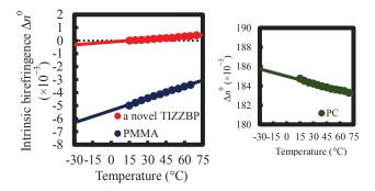
Fig. 2 The relationships between intrinsic birefringence and temperature of a novel TIZZBP, PMMA and PC which degree of orientation *f* at room temperature are 0.15, 0.07 and 0.14, respectively.
