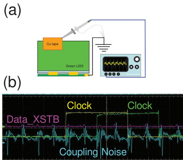
Fig. 1 (a) Illustrates that the measurements of coupling noise. (b) time-domain waveforms of the coupling noise.
