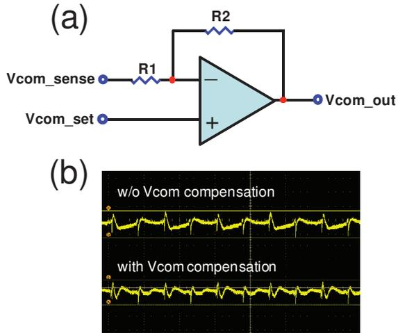
Fig. 2(a) illustrates Vcom compensation circuit. (b) time-domain waveforms of the coupling noise of panel with (gain=150) and without Vcom compensation circuit.
