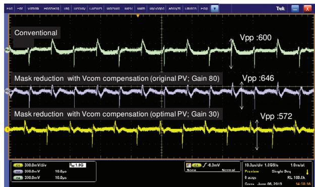
Fig. 5 Comparison of the time-domain waveforms of the coupling noise between the conventional process and mask reduction panel.
