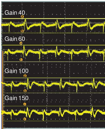
Fig. 3 Time-domain waveforms of the coupling noise of panel at four different gain values.
