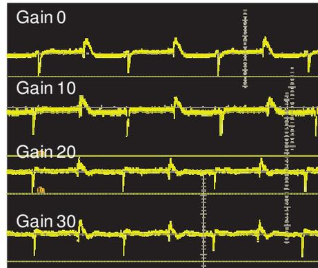
Fig. 4 Time-domain waveforms of the coupling noise of panel with thicker passivation layer at different gain values.
