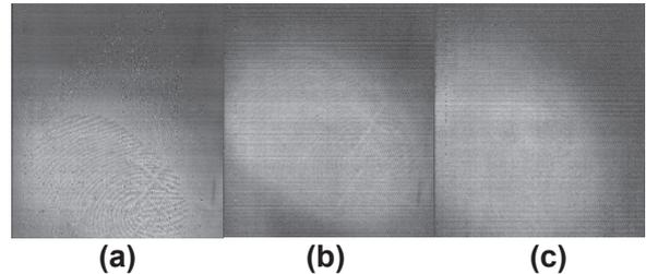
**Fig.5. Different recognition results of IOFPR screen in different states. (a) IOFPR screen without cover glass. (b) IOFPR screen with a thin cover glass. (c) IOFPR screen with a thick cover glass.**
