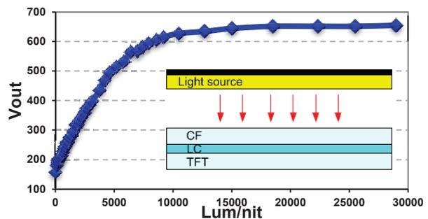
**Fig.3. The sensitivity curve of the IOFPR sensor to the external light source obtained by placing the IOFPR screen under the light source.**
