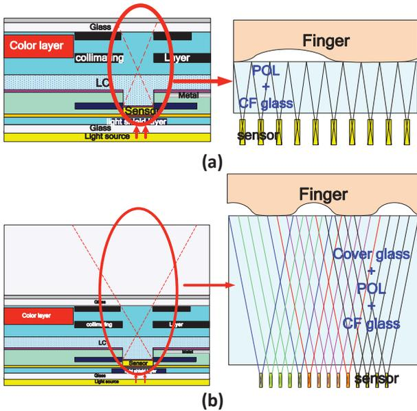
**Fig.4. Different states of IOFPR screen. (a) IOFPR screen without cover glass. (b) IOFPR screen with cover glass.**
