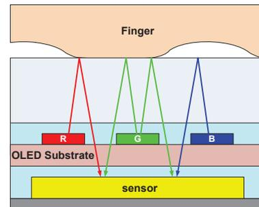
Fig. 1 Under-screen optical fingerprint recognition structure for OLED.
