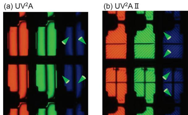
Figure 4. Photographs of white-state (on-state) for (a) UV<sup>2</sup>A and (b) UV<sup>2</sup>A II panels.
