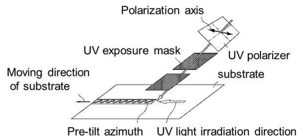
Figure 2. Schematic illustrations of the new UV exposure system for UV<sup>2</sup>A II.
