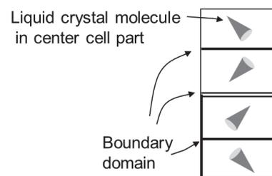
Figure 1. Schematic illustrations of LC orientation for each pixel of UV<sup>2</sup>A II.
