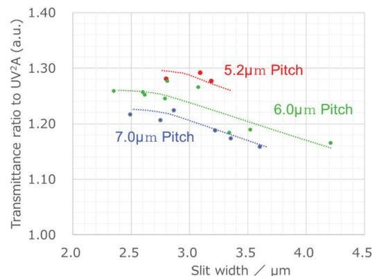
Figure 5. Evaluation results of transmittance ratio to UV<sup>2</sup>A for each slit condition.
