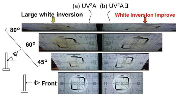
Figure 7. Evaluation results of viewing angle performance; (a) UV<sup>2</sup>A and (b) UV<sup>2</sup>A II.
