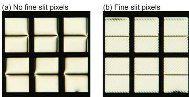
Figure 3. Photographs of white-state (on-state) for UV<sup>2</sup>A II panels of (a) No fine slit pixels and (b) Fine slit pixels.
