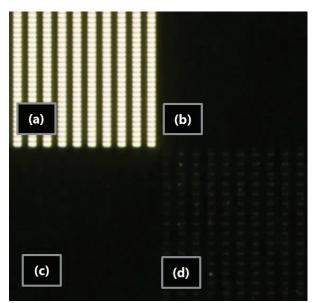
Fig. 4 Optical micrograph of neighbouring pixel areas on the dual cell display driven in different states (a) – both cells fully open, (b, c) – both cells fully closed; (d) – display cell closed, modulation cell open.
