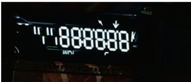
**Fig. 6 A prototype prepared by proposed vertical photoaligned material**
