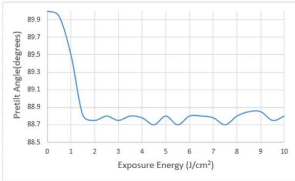
**Fig. 1 Pretilt as a function of exposure energy at 365nm UV light for proposed vertical photoaligned material**
