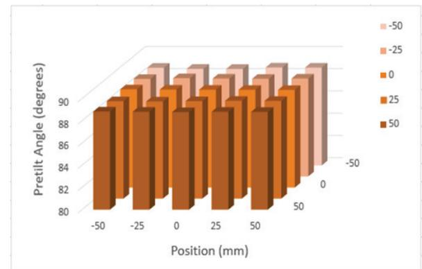
**Fig. 4 Pretilt angle profile in 10cm x 10cm LCD with proposed VA photoalignment using blue LED array exposure**
