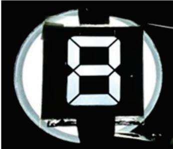
**Fig. 5 A small cell prepared by proposed vertical photoaligned material**
