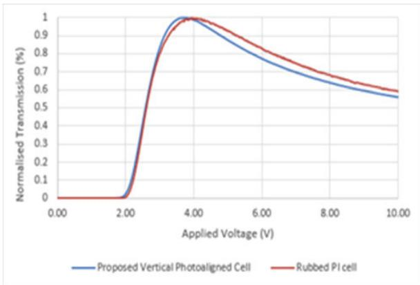
**Fig. 2 TVC curves for proposed vertical photoaligned and rubbed VAN cells.**
