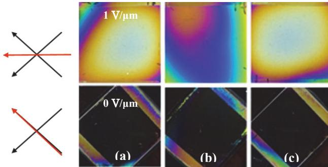
**Fig. 3** The POM photos of UV<sup>2</sup>A LC cells under UV exposure of (a) 11, (b) 14 and (c) 17 sec.
