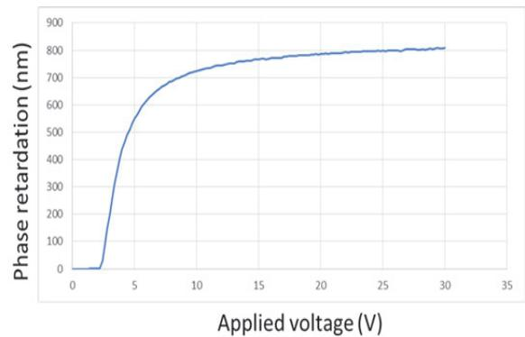
**Fig. 5.** The results of voltage dependent phase retardation dependent of UV<sup>2</sup>A LC cell.
