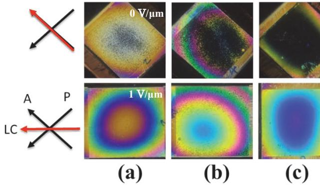
**Fig. 2** The POM photos of UV<sup>2</sup>A LC cells under UV treatment of (a) 2, (b) 4 and (c) 8 seconds.
