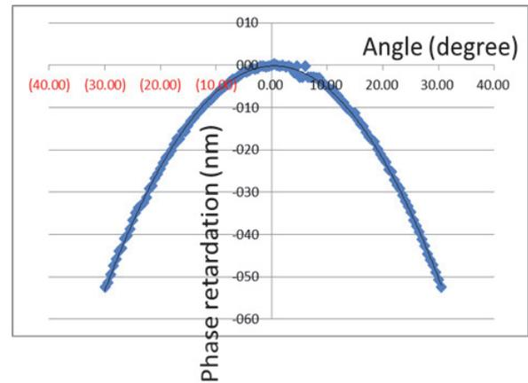
**Fig. 4.** The results of rotation angle dependent phase retardation of UV<sup>2</sup>A LC cell.
