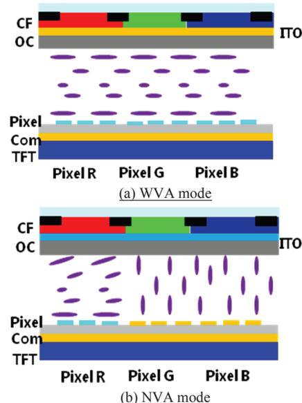
**Fig2. Schematic of the conventional VAC FFS LCD**
