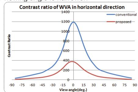
**Fig5. Contrast ratio of both devices of WVA mode in horizontal direction**
