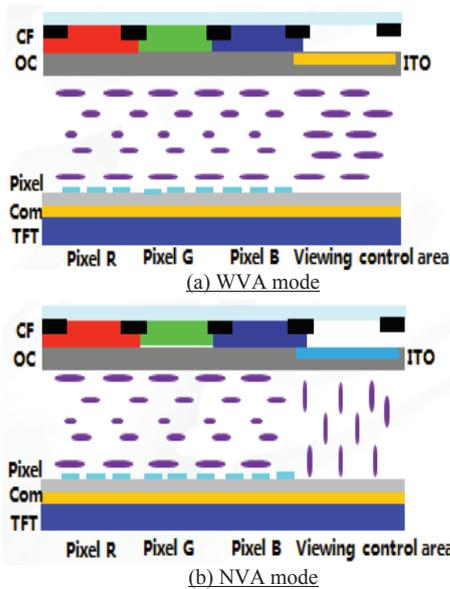
**Fig3. Schematic of the proposed VAC FFS LCD with RGBW CF**
