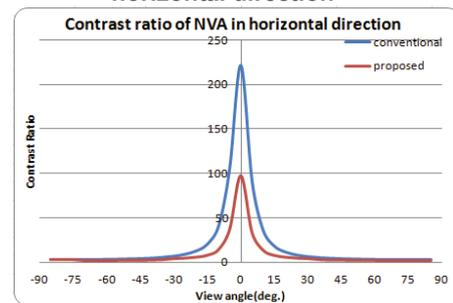
**Fig6. Contrast ratio of both devices of NVA mode in horizontal direction**
