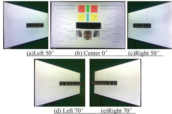
**Fig4. Prototype 13.3inch VAC-LCD of proposed device**
