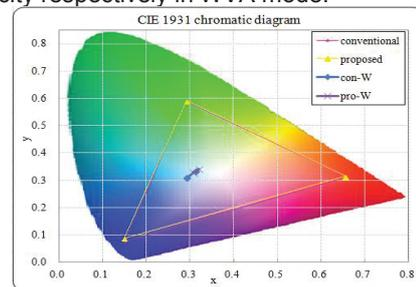
Fig8. Color Chromaticity of the both devices VAC-LCD
