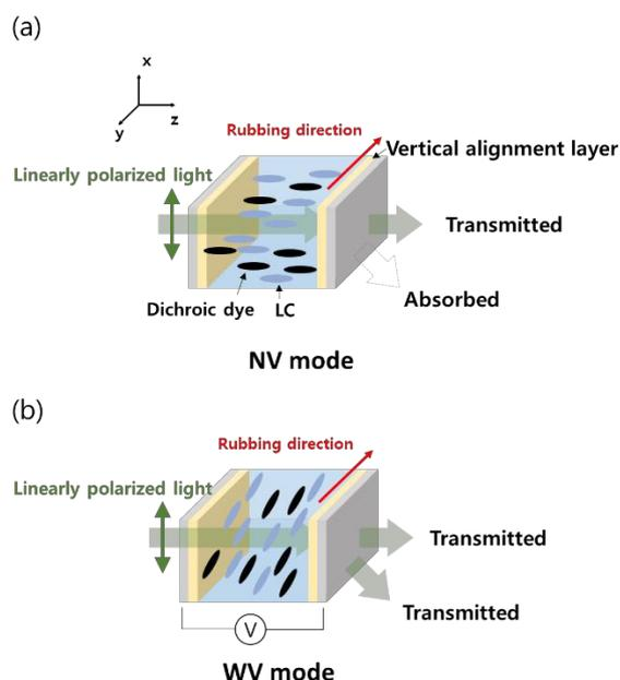
Fig. 1 Schematic illustration of operation principle of the (a) NV and (b) WV mode.
