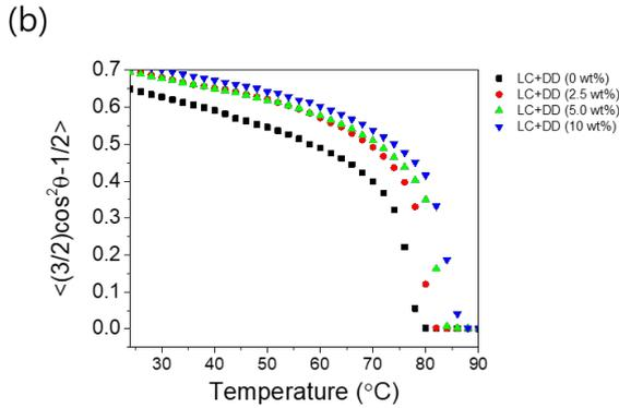
**Fig. 2 (a) The birefringence  $\Delta n$ , (b) order parameter with various concentration of DD vs. temperature  $T$ .**
