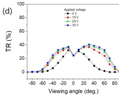
**Fig. 4 Experimental results of the TR vs. horizontal viewing angle. The concentration of the DD in GH cell is (a) 0, (b) 2.5, (c) 5.0, and (d) 10 wt%.**
