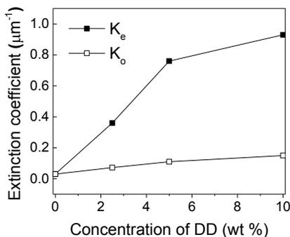
**Fig. 3 Measured results of extinction coefficient vs. concentration of DD.**
